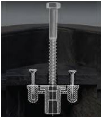
Non-Seizing Bolt System Allows Field Replacement
